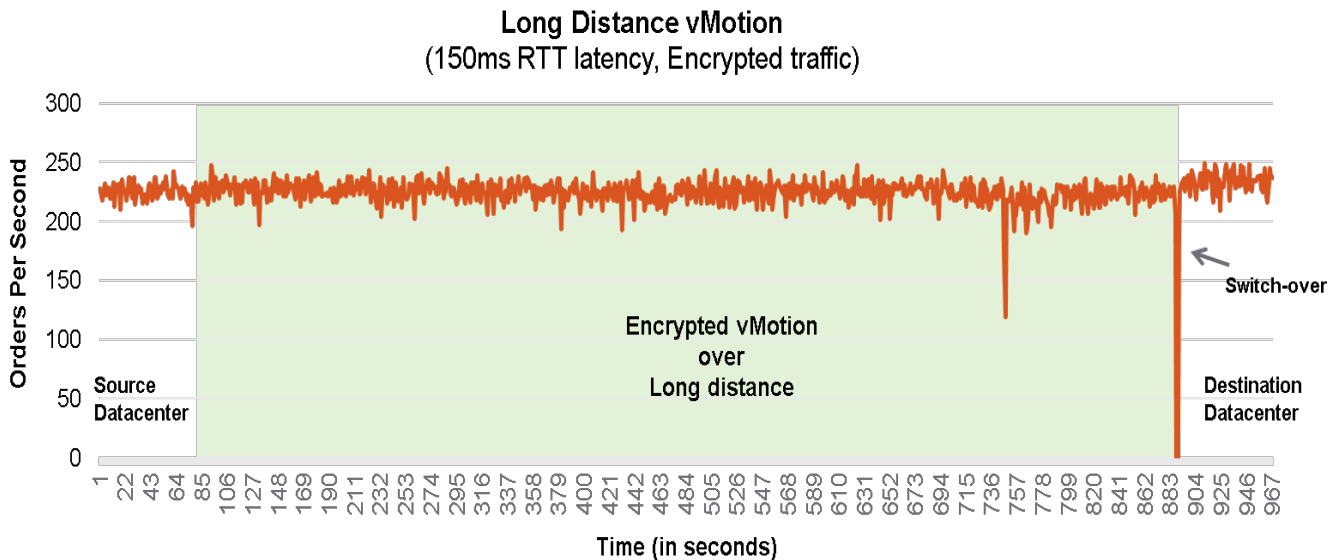
Figure 11. SQL Server performance before, during, and after long distance encrypted vMotion
