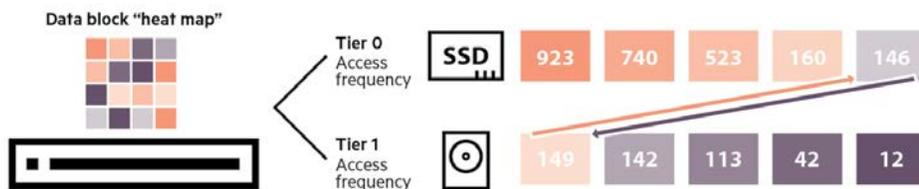
Figure 11. Adaptive Optimization - data balanced dynamically between tiers
